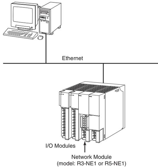
When the R3 Series is used, actual sampling rate depends upon the number of connected devices (nodes) and the number of channels.
