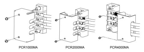
Attach a crimping terminal to the switchboard end of the power cord.
