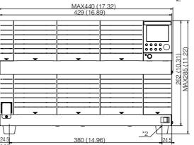
\*1: Eight M4 screw holes (max. depth 8 mm) \*2: Four M4 screw holes (max. depth 8 mm)
