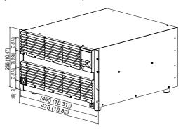
When mounting on a millimeter rack (Bracket model: KRB300)
