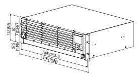
When mounting on a millimeter rack (Bracket model: KRB150-TOS)
