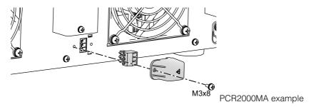
Connect the sensing cables to the connector.
