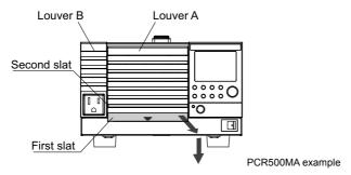
While pressing up on the bottom tab of louver B, pull it towards you. Slide the entire louver down, and remove the louver from the panel.
