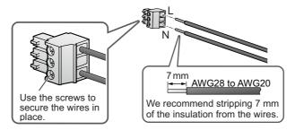
Attach the connector and SENSE terminal cover.
