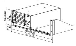
When mounting on a millimeter rack (Bracket model: KRA150)
